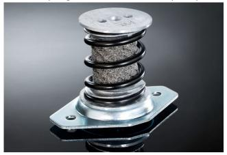
Spring isolators for machine mountings with a natural frequency below 9 Hz are highlighted in yellow. These elements are available in many designs, always depending on the load range and the respective excitation frequency of the system. Standard spring elements are available in the natural frequency ranges 3-4, 5-6 and 7-9 Hz. The load ranges here are in the range of 5 - 42,000 kg per element.
